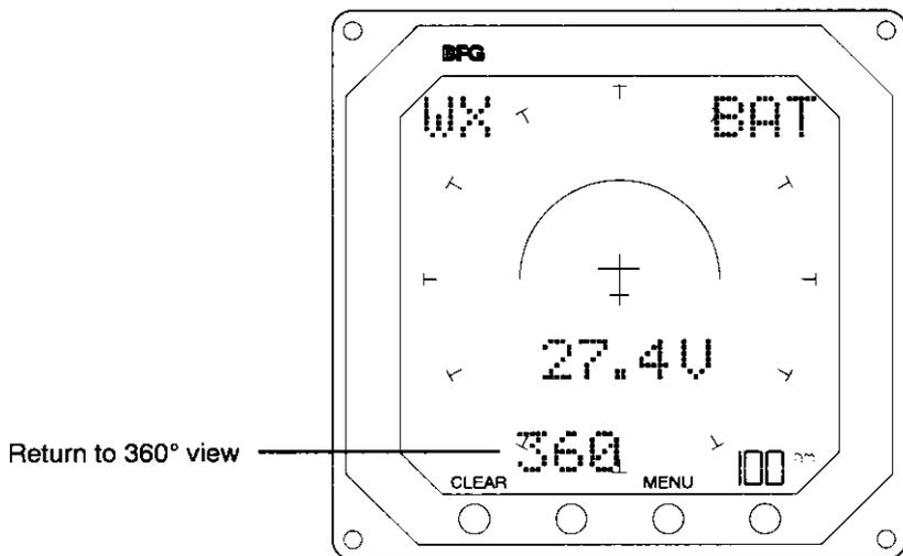
**Figure 1-14: Battery Voltage Monitor Display in Weather Mode**
