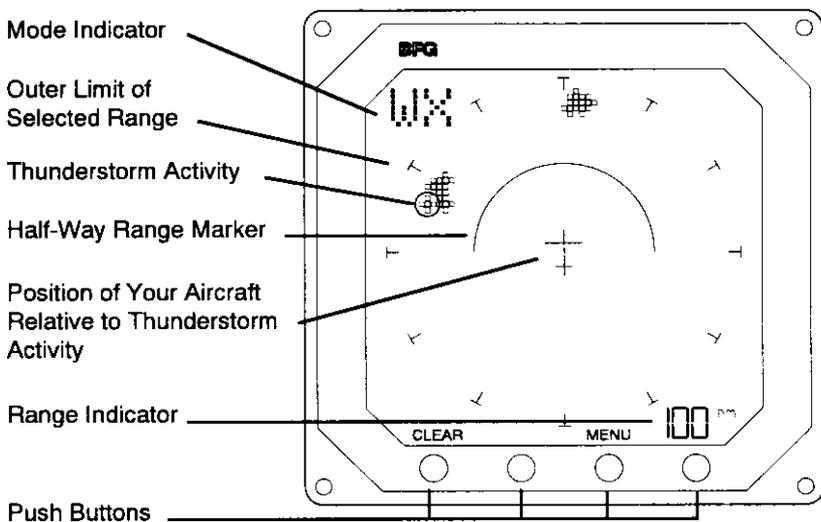
**Figure 1-1: Legends and Controls in Weather Mode**
