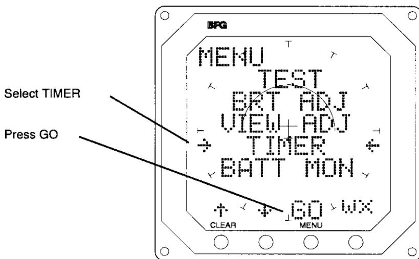
**Figure 1-10: Selecting the Timer Mode from the Mode Menu**
