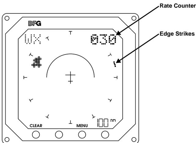
Lightning strikes detected beyond 100 miles will be plotted as a single pixel on the outer range ring at the corresponding azimuth. These strikes, as shown above, are called edge strikes. This information is provided as an aid for longer range planning. Edge strikes are included in the rate counter display.
