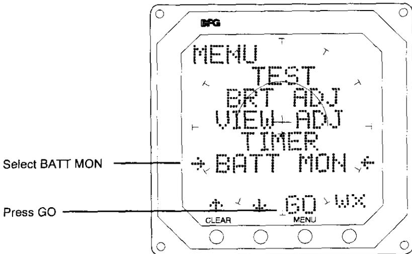
**Figure 1-13: Selecting the Battery Monitor from the Mode Menu**
