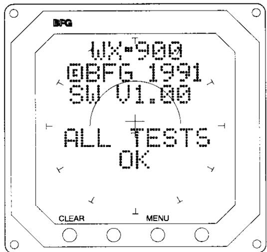
**Figure 1-2: System Start Up Test Completion Message**
