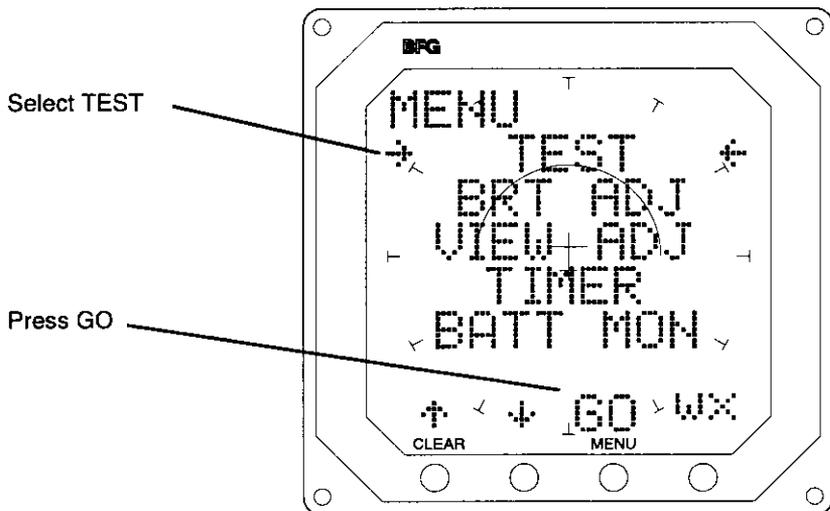
**Figure 1-5: Initiating a User Test from the Mode Menu**
