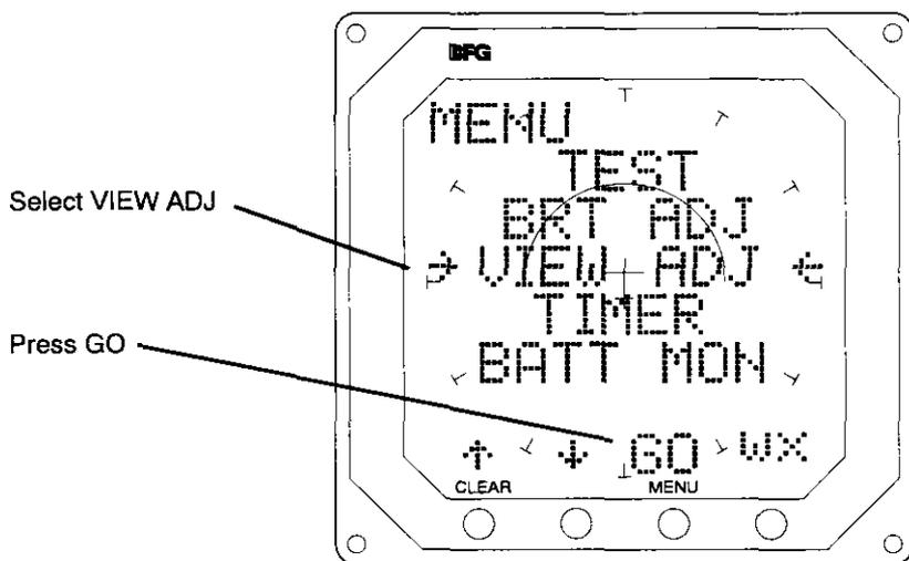
**Figure 1-8: Selecting the View Adjust Mode from the Mode Menu**
